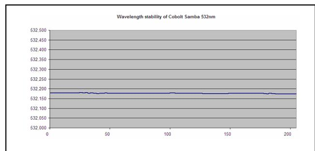
Figure 1: graph showing the long-term wavelength stability of A Cobolt Samba™ 532 nm
